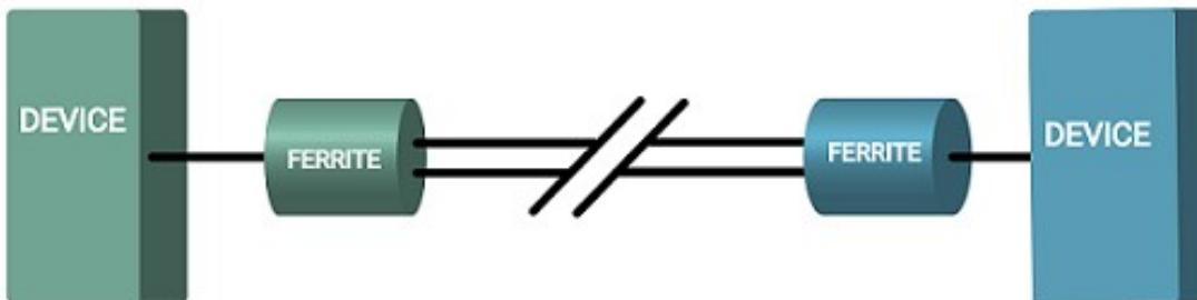
Ferrite used for external cabling
